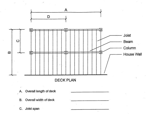
FOOTINGS: If the deck is to be attached to the house, column footings are required for the deck, and the
