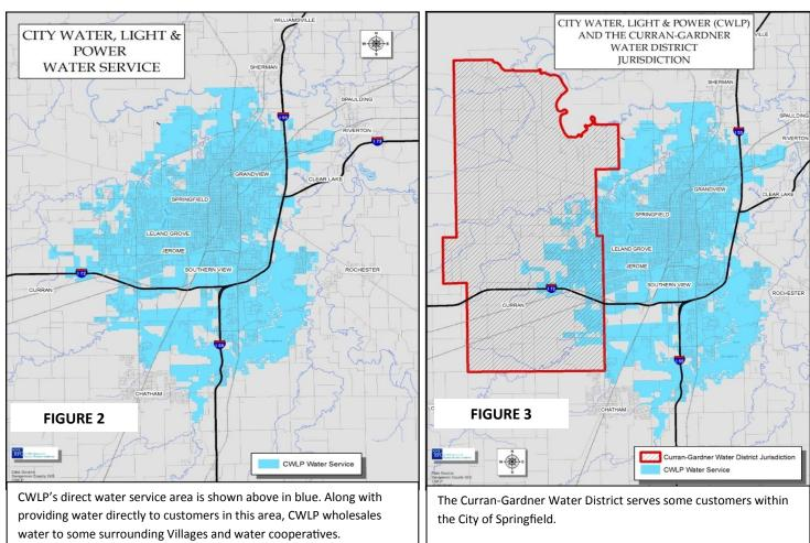
CWLP, the Curran-Gardner district is able to serve customers using CWLP water if it is more practical than extending a new main. CGWD also has a 4" water main connected to CWLP water to provide service in the case of an emergency. CGWD had plans underway to complete an interconnection with the Village of New Berlin water system by the fall of 2016 to provide additional back-up.
